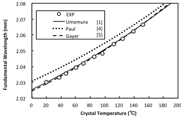
Fig 2. Temperature-dependent wavelengths for QPM / SHG in MgO:PPLN (Λ = 30.8 μm).
