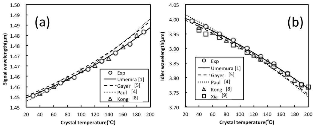
Fig 1. Temperature-tuned signal (a) and idler (b) wavelengths for QPM/OPO (ee-e, m = 1) pumped by a Nd:YAG at 1.0642  $\mu\text{m}$  in MgO:PPLN with a grating period of 29.0  $\mu\text{m}$ .
