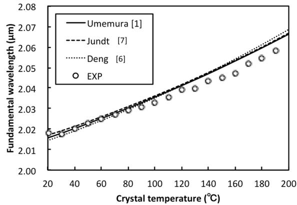
Fig 4. Temperature-tuned fundamental wavelength for QPM/SHG(ee-e,  $m=1$ ) pumped by a Nd:YAG at  $1.0642 \mu\text{m}$  in undoped PPLN with a grating period of  $30.0 \mu\text{m}$ .
