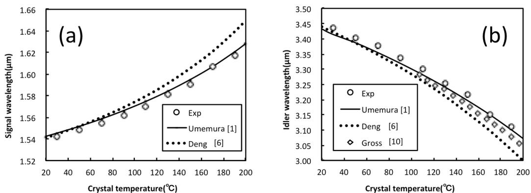
Fig 3. Temperature-tuned signal (a) and idler (b) wavelengths for QPM/OPO (ee-e, m=1) pumped by a Nd:YAG at 1.0642  $\mu$ m in undoped PPLN with a grating period of 30.0  $\mu$ m.
