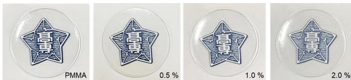
Fig. 4. Optical transparencies of neat PMMA and APC/PMMA nanocomposites containing 0.5, 1.0, and 2.0 wt% APC 2. All samples are around 0.5 mm thick.
