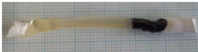
Fig 1. Single-crystals of \text{Lu}_2\text{O}_3\text{-Tb}_2\text{O}_3 , grown by the floating-zone method.
